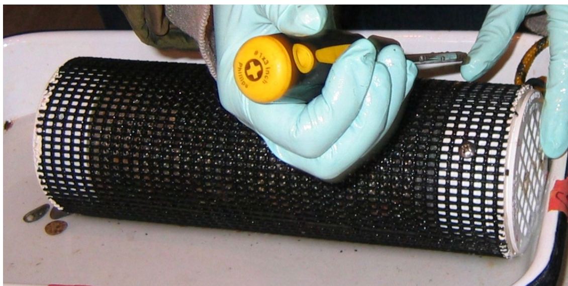
Figure 3.1. Egg tube to house wild chum salmon eggs and alevin while in the artificial redd
